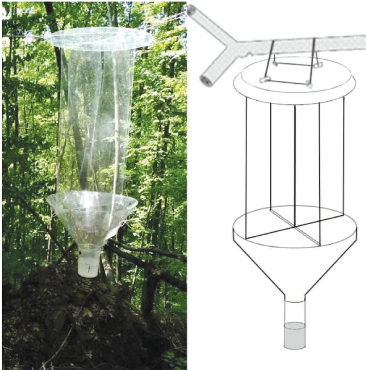
Fig. 2. Scheme and general view of the window combined trap (polytrap).
